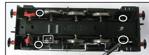
Body removal screws. Marked in square is the cab light on / off switch.
